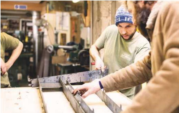
Assembling the custom-sloped frame which will convert the Wadkin thickener into a wedge-nesser
